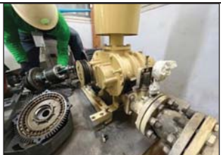
Photo#7 : Inspect & assemble the Air Blower.
