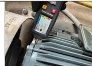
Photo#14 : Check the vibration of the motor.
