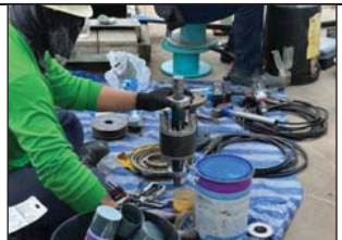
Photo#3 : Change the bearing for Motor.
