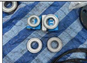
Photo#4 : The motor's new and old bearings.
