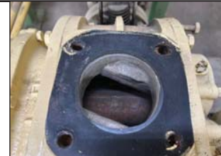
Photo#9 : Rust was found inside the blower. [B-01, (B)]
